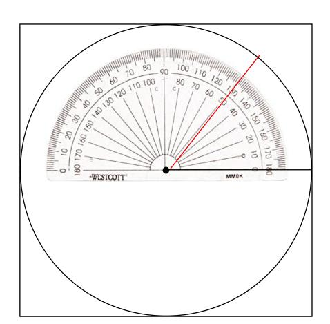
**Step 11 -** Use the new baseline. Set your protractor in the center. Align the protractor to the baseline on the protractor (not the bottom of the protractor!!) Mark the next angle.
