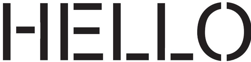
2. Bridge - A thin strip of material that breaks apart larger shapes. Or, a bridge can be used to hold in material to protect negative spaces such as the center of an O shape.
